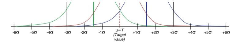
Motorola's, and most industry's interpretation of the six-sigma concept accepts max. 3.4 parts per million to be defective parts, because (as illustrated above), it allows the mean to shift  $\pm$  1.5  $\pm$  around.
