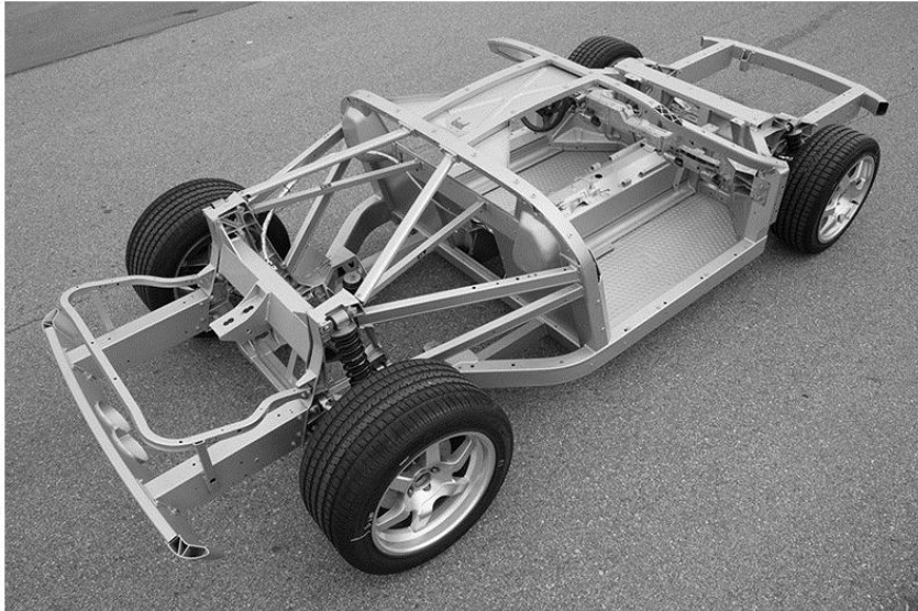
Figure 7-3a) (Left) The space frame chassis for the 2005 Ford GT is comprised of 35 aluminum extrusions, 7 complex castings, 2 semisolid castings, and various aluminum panels, some superplastically formed. (Courtesy Ford Motor, Dearborn, MI; and HydroAluminum of North America Linthicum, MD.)
