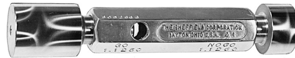
Figure 10-34 Plain plug gage having the go member on the left end (1.1250-in. diameter) and no-go member on the right end. (Courtesy of Sheffield.)
