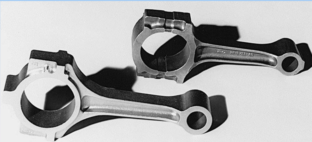
Figure 18-15 P/M forged connecting rods have been produced by the millions. (Courtesy of Metal Powder Industries Federation, Princeton, NJ.)
