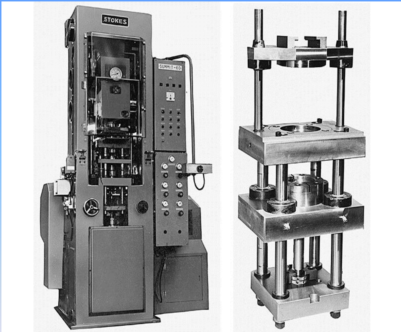
Figure 18-3 (Left) Typical press for the compacting of metal powders. A removable die set (right) allows the machine to be producing parts with one die set while another is being fitted to produce a second product. (Courtesy of Alfa Laval, Inc., Warminster, PA.)
