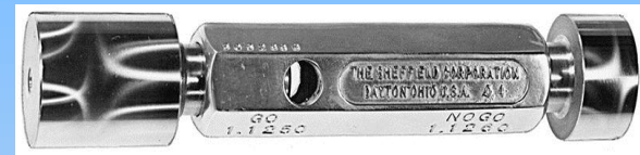
Figure 10-34 Plain plug gage having the go member on the left end (1.1250-in. diameter) and no-go member on the right end. ( Courtesy of Sheffield. )
