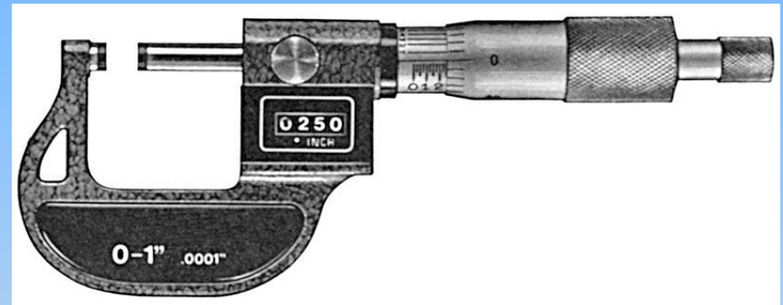
Figure 10-20 Digital micrometer for measurements from 0 to 1 in., in 0.0001-in. graduations.
