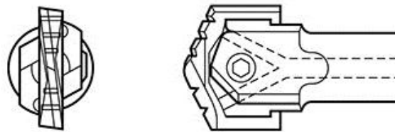
Spade drill with oil holes
