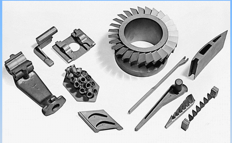
Figure 12-30 Typical parts produced by investment casting. (Courtesy of Haynes International, Kokomo, IN.)
