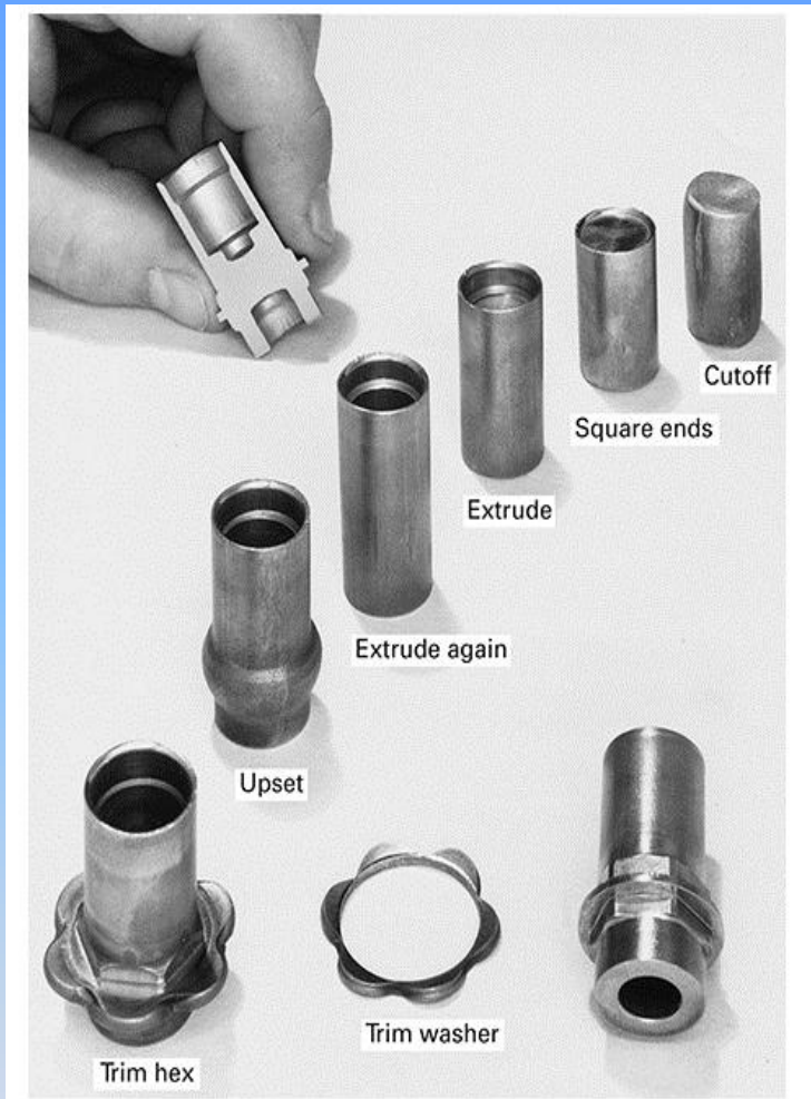
Figure 16-46 Cold-forming sequence involving cutoff, squaring, two extrusions, an upset, and a trimming operation. Also shown are the finished part and the trimmed scrap. (Courtesy of National Machinery Co., Tiffin, OH.)
