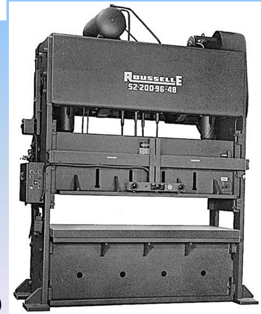
Figure 17-61 (Right) A 200-ton (1800-kN) straight-sided press. (Courtesy of Roussele Corporation, West Chicago, IL.)
