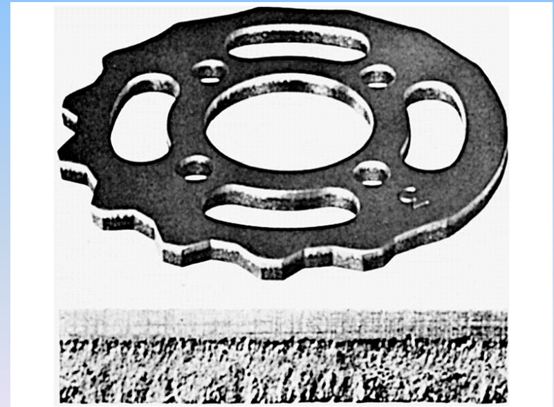
Figure 17-2 (Right) (Top) Conventionally sheared surface showing the distinct regions of deformation and fracture and (bottom) magnified view of the sheared edge. (Courtesy of Feintool Equipment Corp., Cincinnati, OH.)
