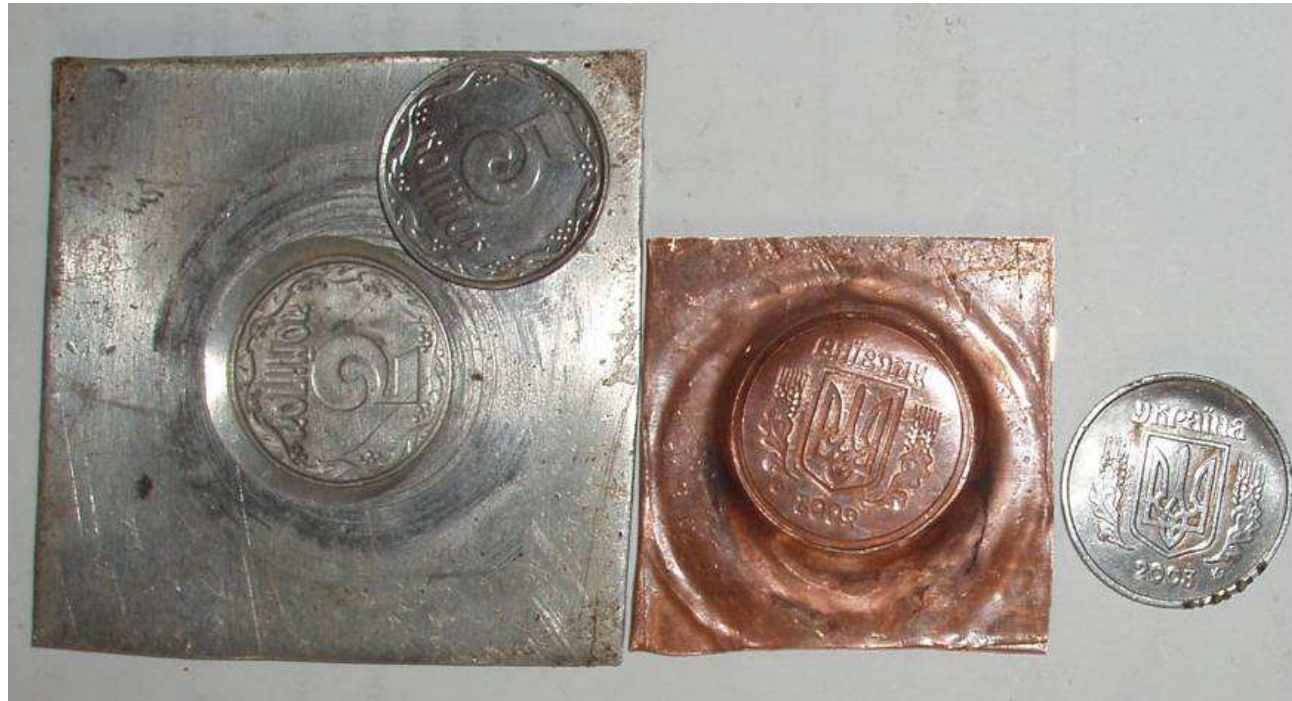
Figure 13. General view of a coin stamped on aluminum and copper samples. Notice reproduction of fine details of the coin on the sample surface.
