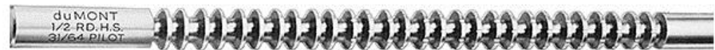
(b) Round, push-type broach with chip-breaking notches on alternate teeth except at the finishing end.
