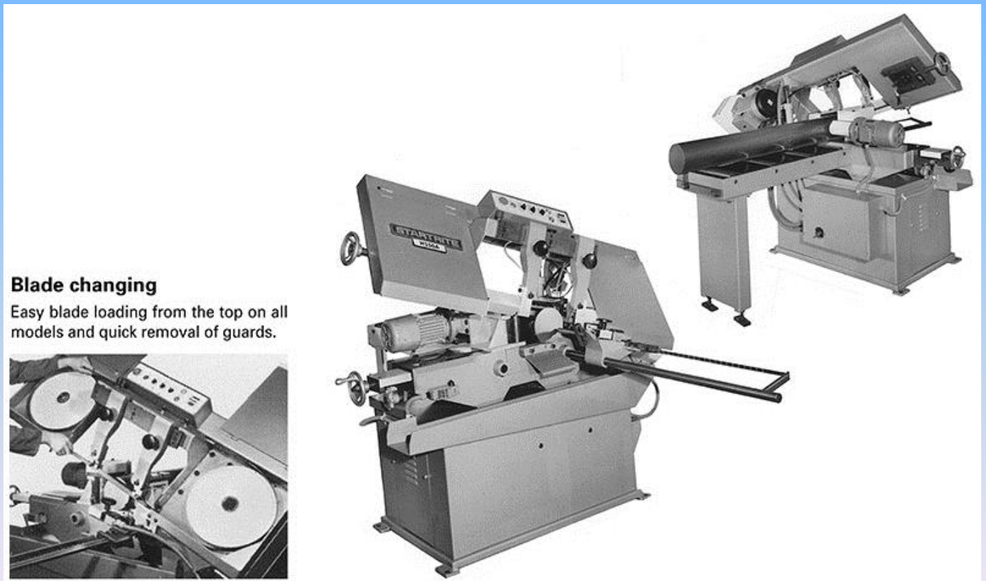
FIGURE 27-16 Front view and rear view of a horizontal bandsawing machine sawing a cylinder of steel. Inset shows blade-changing operation.
